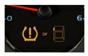
Indirect TPMS – the antilock braking system (ABS) uses wheel speed sensors to measure the rate of revolutions for each wheel. When the system detects that a wheel is spinning faster than expected due to it being under-inflated, it sends an alert to the driver
