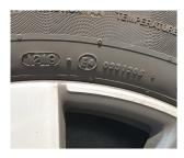
If you buy a retreaded tyre, make sure that it has the E-mark on it, which confirms that a tyre meets minimum EU or International (UNECE) standards in relation to its dimensions, load and speed rating. All motor vehicles tyres in the EU must be E-marked, whether new or retreaded.
