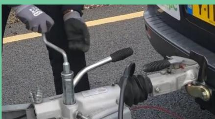
Lower the trailer, using the jockey wheel, until it clicks into place onto the towing ball. When in place, increase the height of the jockey wheel to test that the towing vehicle's rear end raises with it, showing that they are connected securely.
