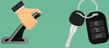
Ensure the vehicle's parking brake is applied, stop the engine and remove the keys. Ensure trailer parking brake is also applied. Carry out a trailer safety check.
