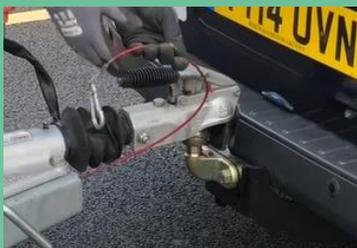
Disconnect the breakaway cable and stow away safely.
